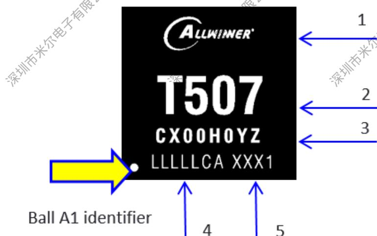
Figure 11-2. T507 CX00H0YZ Marking
