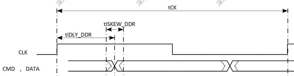
Figure 5-27. SMHC0/1 DDR50 Mode Input Timing Diagram
