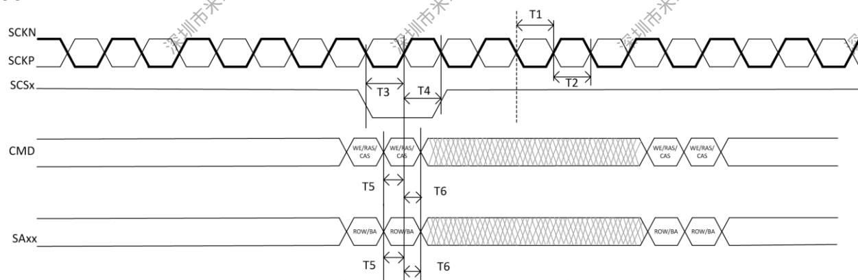
Figure 5-5. LPDDR3 Command and Address Timing Diagram
