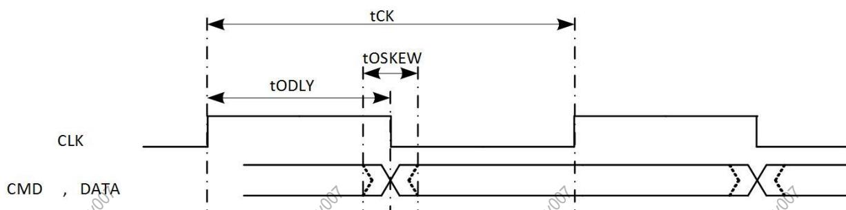
Figure 5-34. SMHC2 HS200 Mode Output Timing Diagram
