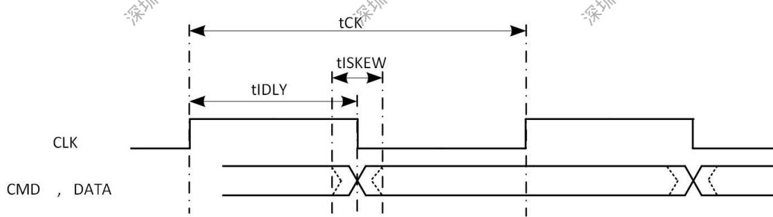
Figure 5-25. SMHC0/1 SDR Mode Input Timing Diagram
