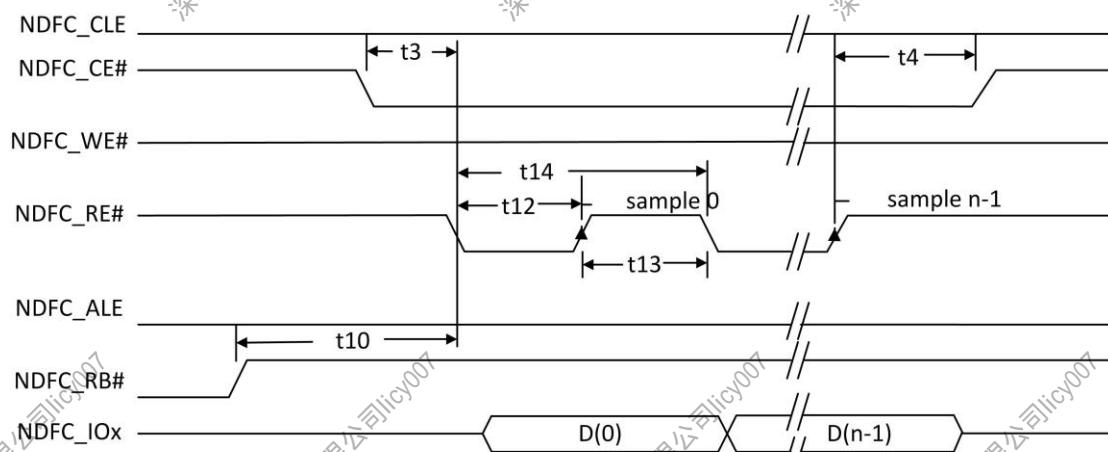
Figure 5-14. Conventional Serial Access Cycle Timing (SAM0)
