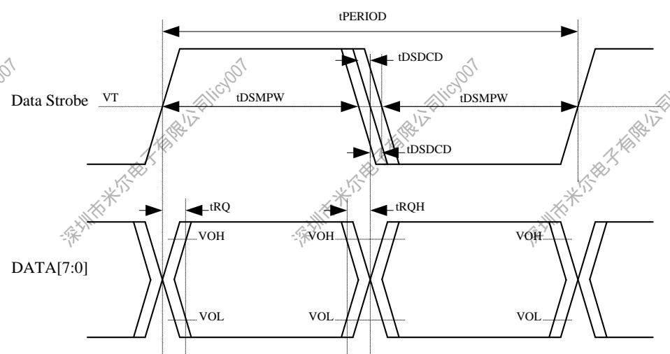
Figure 5-37. SMHC2 HS400 Mode Data Input Timing Diagram
