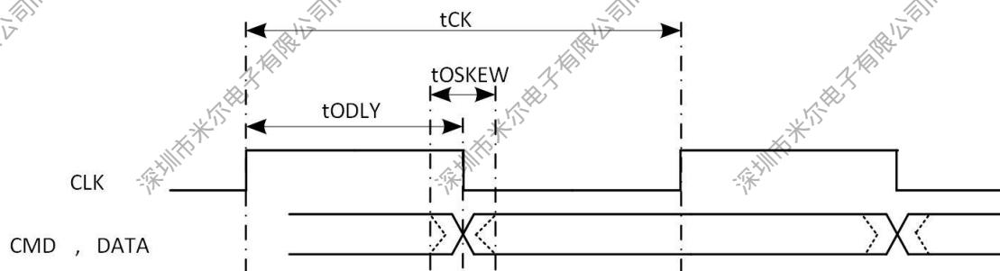
Figure 5-24. SMHC0/1 SDR Mode Output Timing Diagram
