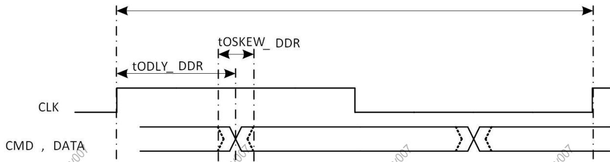
Figure 5-31. SMHC2 HS-DDR Mode Output Timing Diagram
