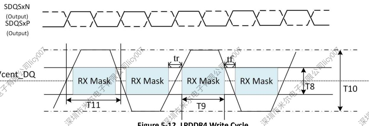
Figure 5-12. LPDDR4 Write Cycle
