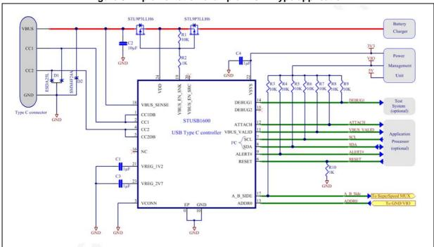
Note: Schematic configuration is in dead battery mode.
