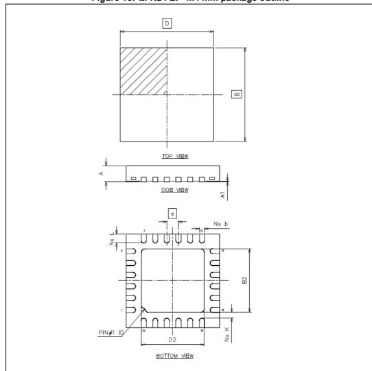
Figure 10. QFN24 EP 4x4 mm package outline
