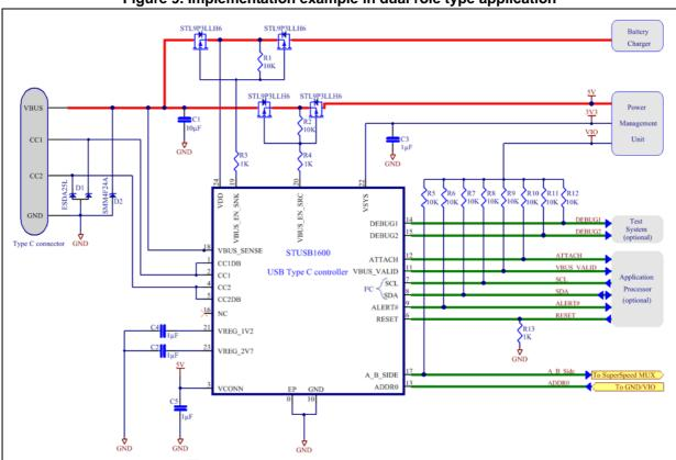
Note: Schematic configuration is in dead battery mode.
