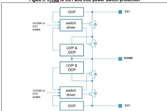
Figure 3. V<sub>CONN</sub> to CC1 and CC2 power switch protection
